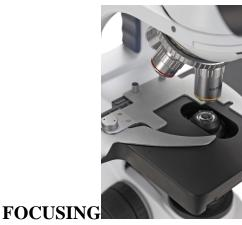
Double coaxial, low-positioned coarse and fine adjustments with 180 graduations. Precision 1.11  $\mu$ m, 200  $\mu$ m per rotation, total travel approximately 19 mm. Supplied with an adjustable rack stop to prevent damage to sample and objectives. The coarse adjustment is equipped with friction control
